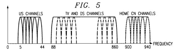
Petitioner asserts that Amit's Figure 5 above shows that the terminal devices have multiple channels ("frequency bins") for terminal devices to use to for transmission. *Id.* at 20–21 (citing Ex. 1001, 8:42–43; Ex. 1005, 5:28–29, 7:61–65).
