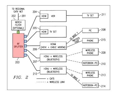
Referring to Figure 2 above, Petitioner asserts that the RF splitter 203 (red) has a common port (green) connected to notch filter 202, and tap ports (blue) connected to devices 204–207, 212. Pet. 16–17 (citing Ex. 1005, 6:36–39; Ex. 1003 ¶ 63).
