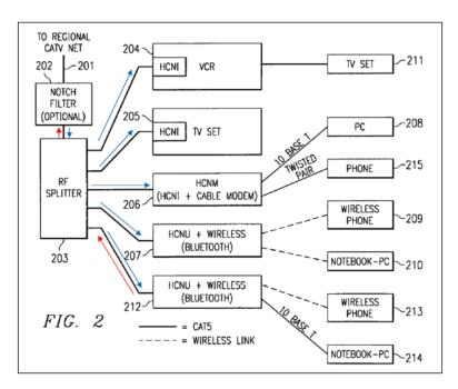
Petitioner annotates Figure 2 to show an exemplary path where HCNU 212 transmits signals through splitter 203 that reflect off filter 202 before passing through splitter 203 again and flowing out each other tap port to terminal devices 204–207. *Id.* at 23–24.
