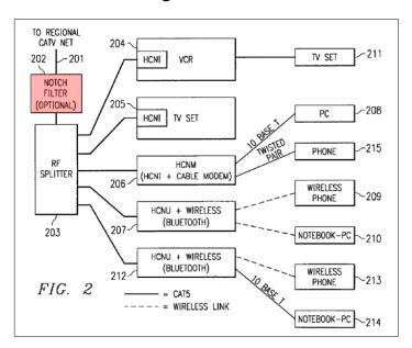
Petitioner annotates Amit's Figure 2 above to highlight the notch filter (red). Petitioner states that this feature of the claimed invention is disclosed, for example, in the following passage of Amit:
