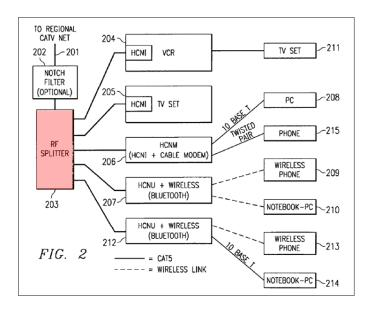
Petitioner annotates Amit's Figure 2 above to highlight RF splitter 203 (red). For example, Petitioner asserts that Amit discloses that "RF splitter [203] splits the signal coming from and to the regional CATV plant [201], to the signals coming to and from units [204–207, 212] respectively." *Id.* at 14 (citing Ex. 1005, 6:36–39). Petitioner further contends that Amit's Figure 7 discloses two splitters 705, 706. *Id.* (citing Ex. 1005, 5:31).
