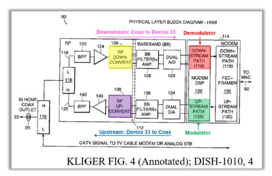
Petitioner's annotated Figure 4 shows that Kliger's HNM includes equivalents of the claimed multi-carrier modulator (green), up converter (purple), down converter (yellow), and multi-carrier demodulator (red).
