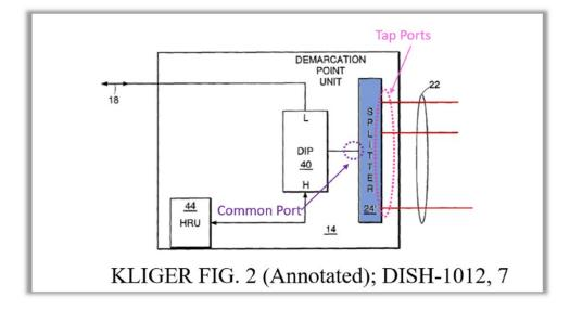
Petitioner's annotated version of Kliger's Figure 2 shows details of demarcation point unit (DPU) 14 including splitter 24 (blue), common port (purple) and tap ports (pink) connected to coaxial cable segments (red).
