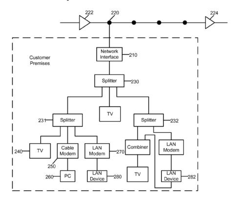
Figure 2 depicts "a signal distribution plan" of the '518 patent. *Id.* at 5:12–13. LAN modem 270 modulates and demodulates a waveform transmitted over the cable, and has an interface to communicate with LAN
