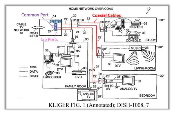
Petitioner's annotated Figure 1 shows segments of coaxial cables (red) and the demarcation point unit's splitter 24 (blue) with common port (purple) and tap ports (pink).
