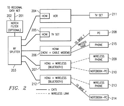
Figure 2 shows Home Cable Networking (HomeCN/HCN) having five home networking devices (also called "nodes" or "home units") 204–207 and 212 connected to a regional CATV plant via cable 201. *Id.* at 2:13–17, 4:23–24, 6:24–26. Amit's nodes include a VCR 204 and TV Set 205 with Home Cable Networking Interfaces (HCNI). *Id.* at 6:44–46. Amit's nodes further include Home Cable Networking Modem (HCNM) 206, and Home Cable Networking Units (HCNUs) 207, 212. *Id.* at 6:3–23.
