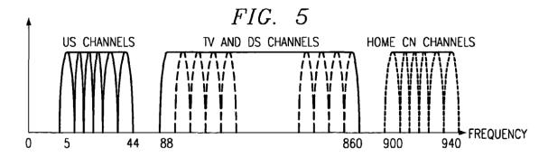
Figure 5 shows Amit's frequency allocation. Ex. 1014, 5:28–29. Petitioner asserts that, as shown in Amit's Figure 5, the frequency band used by cable television service is below 860 MHz whereas the frequency band dedicated to the HomeCN channels, the claimed "RF carrier frequency," is 900–940 MHz and thus is "above the frequency used by the cable television service" as claimed. Pet. 81 (citing Ex. 1014, 7:61–8:3, 8:22–28, Fig. 5; Ex. 1004 ¶¶ 273–277).
