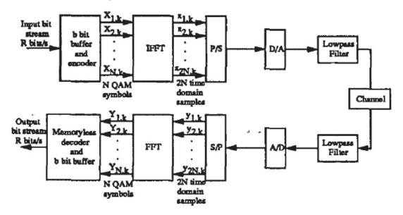
The components in the upper part of Jacobsen's Figure 1 constitute a DMT transmitter, and components in the lower part constitute a DMT receiver. *Id.* at 10.
