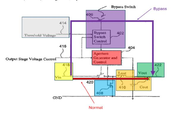
Figure 4, annotated by Petitioner, shows both the normal pathway (red) and bypass pathway (purple).
