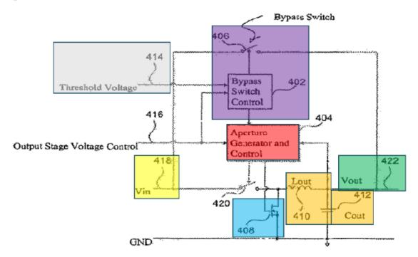
Figure 4, annotated by Petitioner, illustrates "an example step down switching power supply having a bypass switch architecture." Ex. 1001, 3:5–6. As shown in Figure 4, power supply 400 receives an "input voltage signal"  $V_{IN}$  418 (yellow), an "Output Stage Voltage Control signal" 416, and a "Threshold Voltage signal" 414 (grey). *Id.* at 6:38–40.
