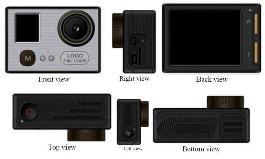
The photo on the top row left is a "front view" of the claimed camera, the photo on the top row middle is a "right view," the photo on the top row right is a "back view," the photo on the bottom row left is a "top view," the photo on the bottom row middle is a "left view," and the photo on the bottom row right is a "bottom view."
