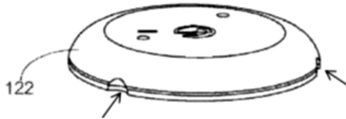
Annotated Figure 17 (detail) of the '335 patent, indicating with arrows the plurality of recesses on the periphery of the on-body electronics housing unit 122
