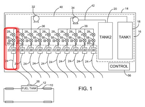
According to Permian, annotated Figure 1 "shows that the reels 30 are fluidly connected to the hoses [24] and manifolds [36, 38]" and one skilled in the art "would have understood, *based on this diagram* . . . that the reel 30 is part of the fluid stream, and, therefore, the flow passage passes through the reel." Pet. 27–29 (emphasis added).
