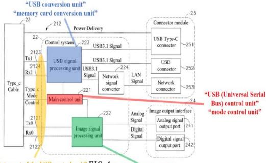
"first data port of the USB control unit" FIG. 4 "mode conversion unit"
