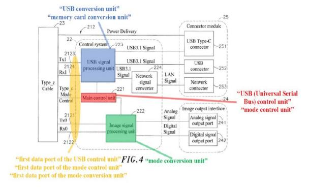
Pet. 79. As annotated Figure 4 of Kuo above shows, control system 22 teaches the DTCM, main control unit 221 (red) teaches the USB control unit and mode control unit, USB signal processing unit 223 (blue) teaches the USB conversion unit and the memory card conversion unit, and image signal processing unit 222 (green) teaches the mode conversion unit. *Id*.
