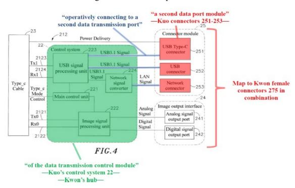
Annotated Figure 4 of Kuo above shows a docking station. Petitioner asserts that Kuo's connectors 251–253 (red) electrically connect (blue lines) to control system 22 (green) via respective ports of control system 22. *Id.* at 31. Petitioner contends that Kuo discloses that control system 22 has main control unit 221, network signal converter 224, and USB signal processing unit 233, controlling data transmission between connectors
