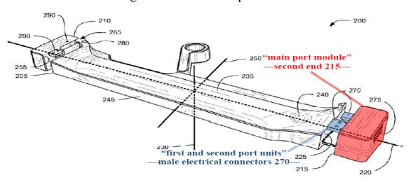
Annotated Figure 2 above shows a docking station. System 200 comprises crossbeam 205 connected to first end member 210 and second end member 215 (red) that includes connectors 270 (blue). Ex. 1005, 5:2–4, 6:44–7:24.
