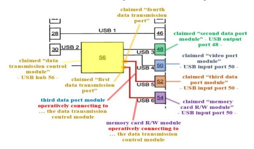
Pet. 75. As shown in annotated Figure 1 of O'Shea above, the combined system would include: a third data port module (brown) operatively connecting (first red line) to a fourth DTP (dark yellow); and a memory card module (purple) operatively connecting (second red line) to a data read/write port (dark yellow) of the DTCM (light yellow) so that a memory card connects to the laptop via the memory card module and the DTCM. Pet. 75.
