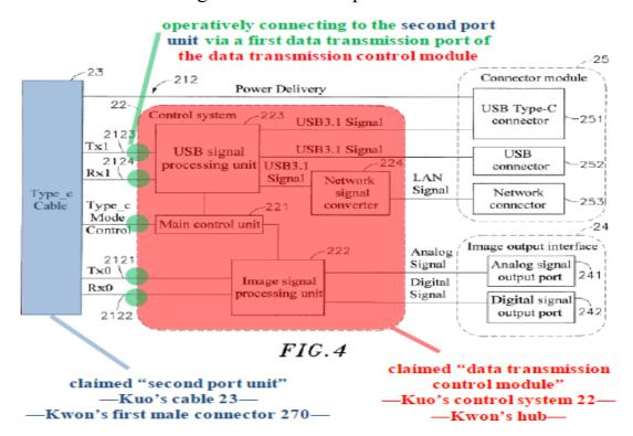
Pet. 23. Annotated Figure 4 of Kuo above shows a circuit block diagram of the electrical module of the docking station. Ex.  $1006 \, \P \, 16$ . Petitioner asserts that control system 22 (red) controls data transmission between peripheral devices connected to output interface ports 24, 25 and cable 23 (blue) for the host computer. Pet. 23 (citing Ex.  $1006 \, \P \, 21$ ; Ex.  $1003 \, \P \, 59$ ).
