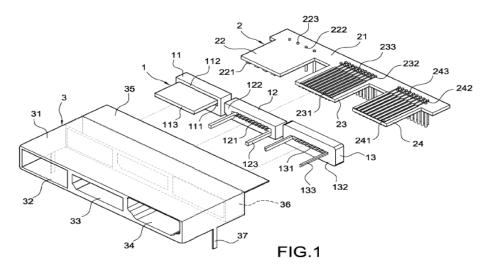
Figure 1 of Chang above illustrates a connector. Ex.  $1008 \, \P \, 25$ . Casing 3 surrounds a plurality of housings 1, which accommodate tongue plates 22-24 of circuit board 2. *Id.* Tongue plate 22-24 of circuit board 2 provide a USB port, a display port, and a HDMI port. *Id.*  $\P \, 37$ . Housings 1 insulate the ports and have perforations 111, 121, 131 for receiving and supporting
