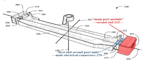
Figure 2 of Kwon above shows docking station system 200 comprising crossbeam 205 connected to first end member 210 and second end member
