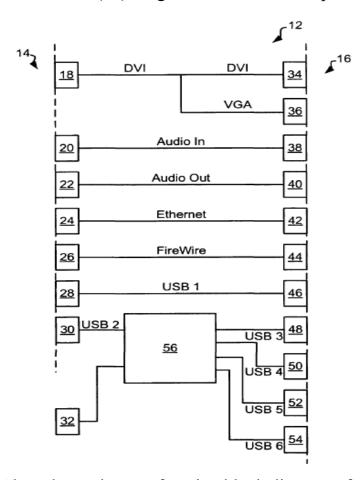
Figure 1 of O'Shea above shows a function block diagram of a connector device. *Id.* at 2:54–56. Connector device 16 includes eight input ports 14 and eleven output ports 16. *Id.* at 2:57–58. Input ports 14 include mini-DVI port 18, audio input port 20, audio output port 22, Ethernet port 24, FireWire
