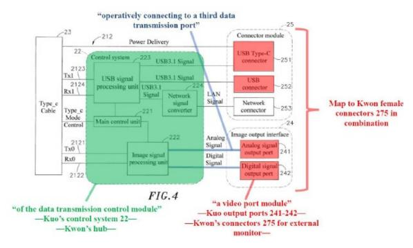
Annotated Figure 4 of Kuo above shows a docking station. Petitioner asserts that Kuo's video ports 241, 242 (red) (video port module) connect (blue lines) to image signal processing unit 222 of control system 22 (green) (DTCM) via respective ports of control system 22. *Id.* at 34 (citing Ex. 1006 ¶¶ 21, 23). Petitioner contends that main control unit 221 and image signal processing unit 222 receive and process to-be-displayed video information.
