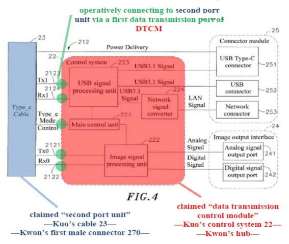
Pet. 23. Annotated Figure 4 of Kuo above is a circuit block diagram of the module of the docking station. Petitioner relies on Figure 4 of Kuo to show that (1) Kuo's control system 22 (red) controls data transmission between peripheral devices connected to output interface ports 24, 25 and cable 23 (blue) for the host computer; and (2) Kuo's channels 2121–2124 (green)
