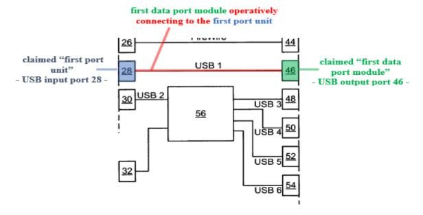
Annotated Figure 1 of O'Shea above is a simplified function block diagram of a connector device. As shown above, USB input port 28 (blue) of O'Shea is directly connected (red) to USB output port 46 (green). Petitioner notes that O'Shea states that "USB port 28 is electronically coupled in a conventional manner to USB port 46 to provide a USB transmission path between the ports." *Id.* (citing Ex. 1007, 4:15–19; Ex. 1003 ¶ 124).
