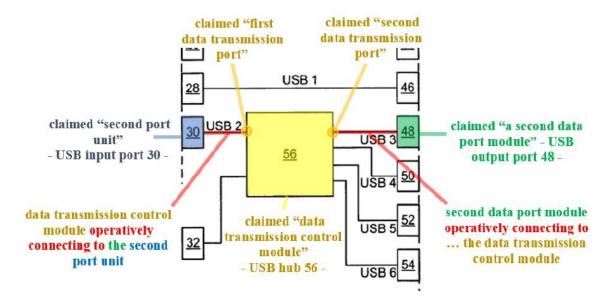
Annotated Figure 1 of O'Shea above shows USB hub 56 (DTCM) (yellow) connected to USB input port 30 (second port unit) (blue) via USB 2 line (first DTP) (red). Petitioner asserts that O'Shea's hub 56 is a DTCM because it is "a conventional device that allows many USB devices to connect to port [30] via ports 48-54." *Id.* at 68 (alteration by Petitioner) (citing Ex. 1007, 4:20–28, 2:57–3:15, 4:35–38; Ex. 1003 ¶ 126; Ex. 1011).
