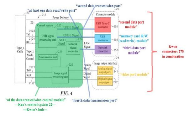
As shown in annotated Figure 4 of Kuo above, the system includes a third data module (connector 253) (purple) operatively connecting to a fourth DTP (third dark blue line) of the DTCM (control system 22) (green), as well as a memory card module (light blue) operatively connecting to a data read/write port (second dark blue line). *Id*.
