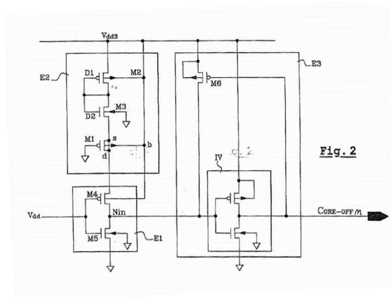
Figure 2 shows a detection device “compris[ing] an output stage E3 following the input stage E1, to obtain the desired output levels for the inverse detection signal CORE-OFF<sub>n</sub>.” Ex. 1008 ¶¶ 35–37.
