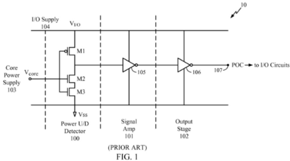
Figure 1 “is a circuit diagram illustrating a conventional POC system for multiple supply voltage devices” which is identified as being prior art. *Id.* at 4:18–19, Fig. 1.
