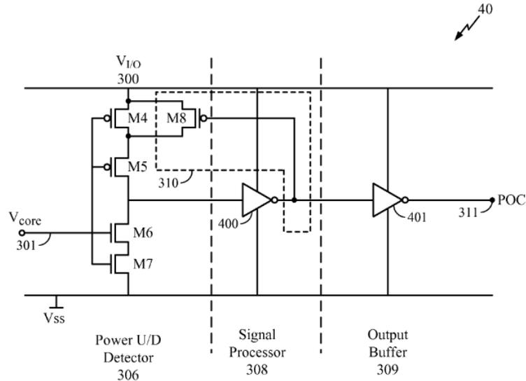
Figure 4 “is a circuit diagram illustrating another POC network configured according to the teachings of the present disclosure.” *Id.* at 4:28–30. The '674 patent describes the operation of the feedback circuit in Figure 4 as follows:
