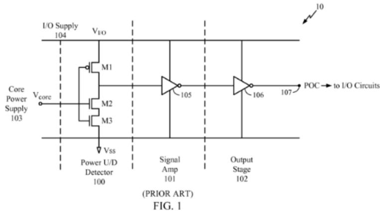
*Id.* at Fig. 1. “FIG. 1 is a circuit diagram illustrating a conventional POC system for multiple supply voltage devices” and is identified as prior art. *Id.* at 4:18–19, Fig. 1. According to the ’674 patent, the POC “is made up of three functional blocks: power-up/down detector 100, signal amplifier 101, and output stage 102. Power-up/down detector 100 has PMOS transistor M1 and NMOS transistors M2-M3.” *Id.* at 1:60–63.
