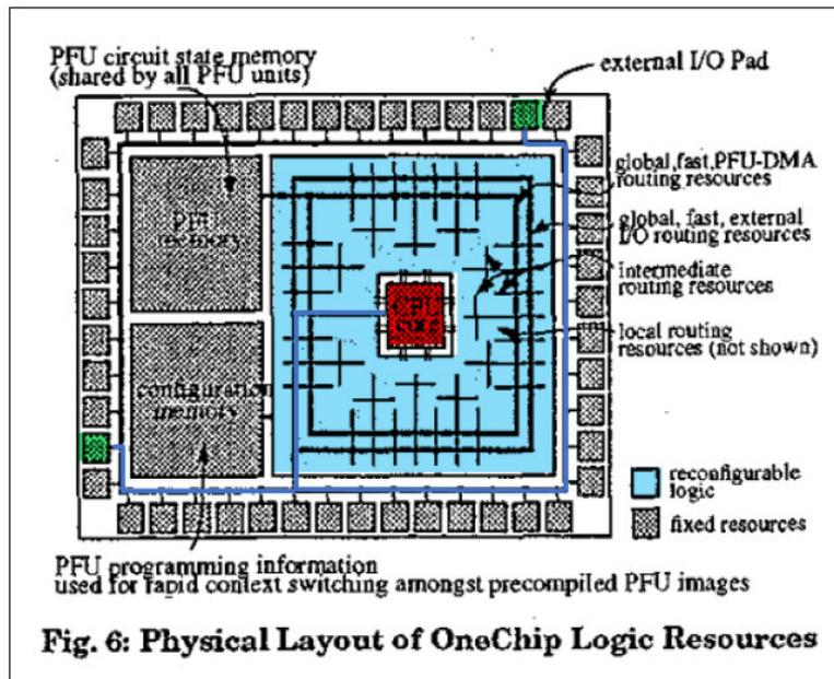
The figure above is a Petitioner-colored version of Figure 6 of OneChip. Pet. 20. The figure shows the physical layout of OneChip’s logical resources, including a CPU (red) surrounded by reconfigurable logic (blue) and having configuration memory (bottom, left), all surrounded by
