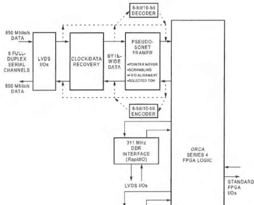
The figure is a portion of a block diagram of the ORT8850 FPSC. *Id.* It includes an LVDS (low voltage differential signaling) input/output (I/O), and a high speed interconnect (HSI) interface to ORCA series 4 FPGA logic. *Id.* A block diagram of the HSI is shown in Figure 3, which is reproduced below. *Id.* at 18–19.
