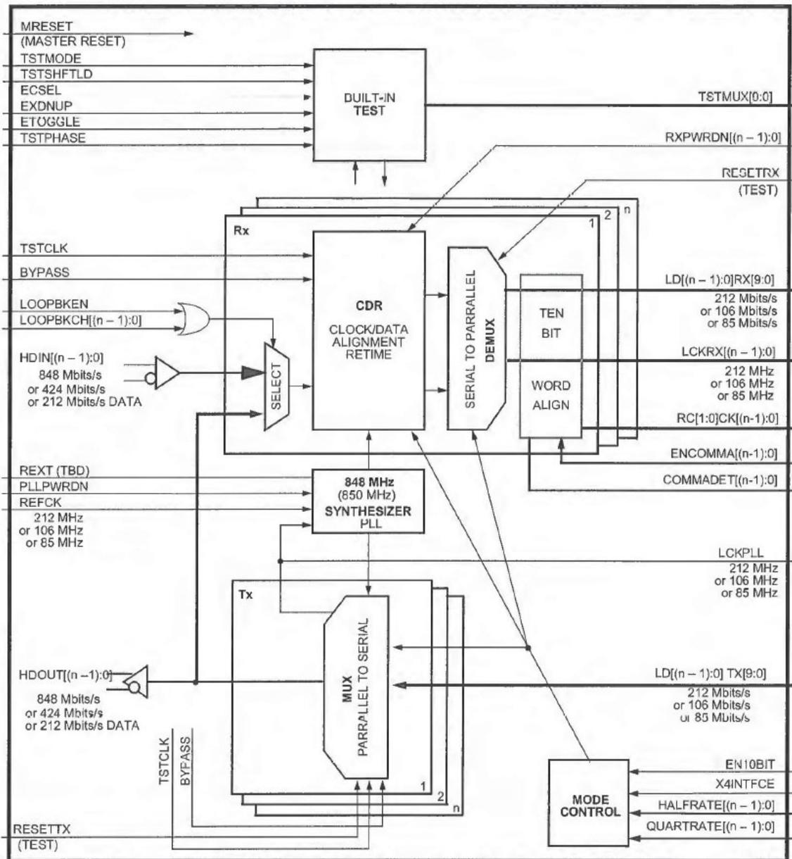
The figure above is Figure 3 of ORT8850, which is an HSI Functional Block Diagram. *Id.* at 19, Fig. 3. For each of n channels, the HSI interface
