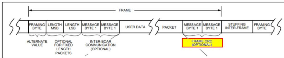
The figure above is a Petitioner-colored version of Figure 6 of an ORT8850 Application Note. Ex. 1015, 6, Fig. 6. As shown in the figure, a frame that is transmitted/received by an ORT8850 transceiver can contain *optional* CRC verification information. *Id.*, Fig. 6. Thus, ORT8850's CRC generator and verification blocks can be optionally used or bypassed depending on whether optional CRC information is included in a transmitted frame or available to be checked in a received frame.
