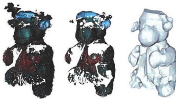
Figure 17: Robustness of the volumetric diffusion tool. Left: The furred object surface produces severe noise and outliers. Center: After the outlier removal, only little object points are left. Right: The volumetric diffusion tool still reconstructs a water-tight model.
