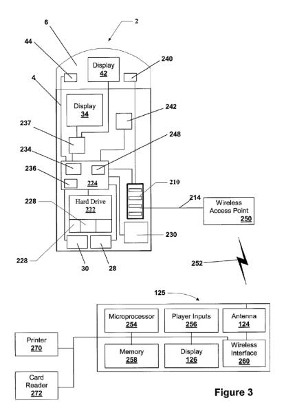
Figure 3 is a block diagram of the internal components of gaming machine 2 and wireless game player 125. *Id.* ¶ 76. "The master gaming controller 224 may communicate with the wireless game player 125 via a wireless communication link 252." *Id.*
