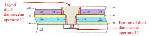
Pet. 44 (annotating Ex. 1003, Fig. 2). The annotations include labels for the top and bottom of aperture 11 (shown in red). *Id.* Similar annotated figures appear in connection with the other instances of the phrase Petitioner seeks to replace. *See* Pet. 57 (mapping the claim language to a combination of Peng modified by Chien<sup>4</sup> and Brase<sup>5</sup>), 84–85 (mapping the claim language to a combination of Lin<sup>6</sup> modified by Chien).
