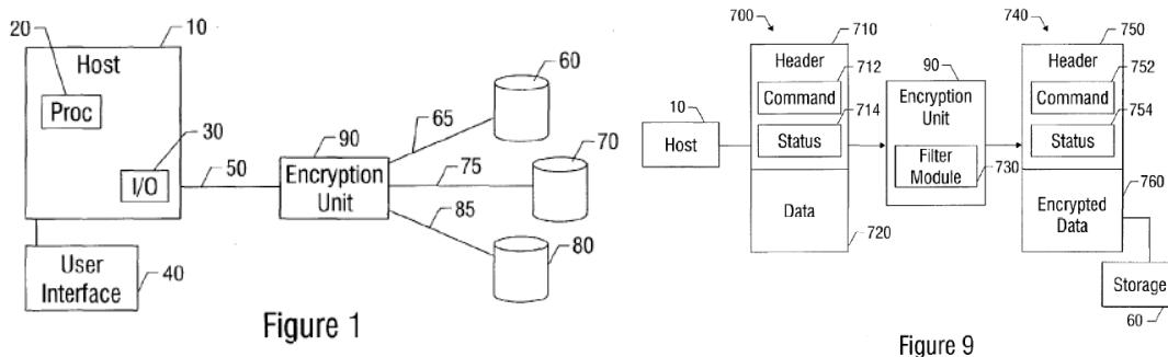
Figure 1 depicts processor-based system 10, which includes subsystem 30 in communication with serial channel or bus 50. Ex. 1002 ¶ 21. Sullivan discloses “[t]he serial channels . . . may be any of a number of other suitable serial channels, such as serial ATA.” *Id.* ¶ 38. Storage devices 60–80 are
