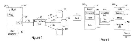
Figure 1 depicts processor-based system 10, which includes subsystem 30 in communication with serial channel or bus 50. Ex.  $1002 \ \mbox{\ } 21$ . Sullivan discloses "[t]he serial channels . . . may be any of a number of other suitable serial channels, such as serial ATA." *Id.*  $\ \mbox{\ } 38$ . Storage devices 60–80 are
