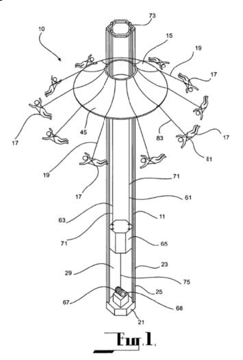
According to the '103 patent, Figure 1 illustrates aerial amusement ride 10, involving conveyance of riders through the air in a manner simulating flight at an elevation sufficiently high to produce a thrilling sensation. *Id.* at 4:58–62. Aerial amusement ride 10 comprises tower 11
